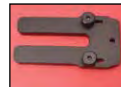
Jims Piston Support Plate provides a non-marring flat support to push the bottom of the piston as rings and cylinder are installed over piston. VT No. 16-1164
