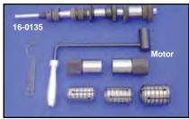
Lapping Tools used for precision alignment of engine and transmission shafts. Engine unit replaces 96710-40 to lap right and left crankcase races for oversized bearings. Transmission tool insures proper fitting of oversized rollers with mainshaft races on Big Twin and Sportsters. The dual-purpose "Combo Lap" for both engine and transmission is also available. Rod laps not
