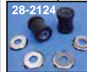
Handlebar Damper Kit consists of one pair of damper, spacers, top and bottom washers. Replaces 56153-73, 46159-73. Fits 1973-84 XL-FX-FL.
