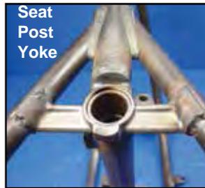
**V-Twin Swingarm Frames** are our authentic reproductions of FLH styles for the years listed to accept Panhead or Shovelhead engines, 4 Speed Transmissions, seat posts and round or square swing arms. Details include forged parts as original in neck, engine mounts, front transmission mount, top seat post yoke, strut and swingarm pivot mount and footboard mounts, as required. All stamped components are pressed and formed as stock.
