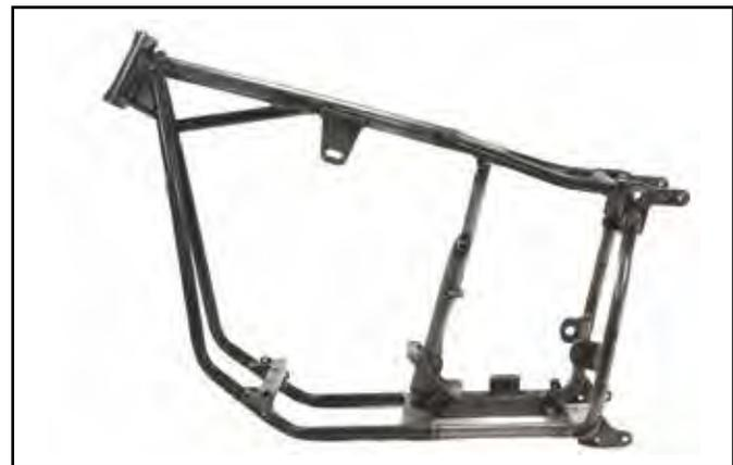
**Paughco Swingarm Frame** accepts Panhead or Shovelhead engines with chain or belt drive. Swingarm frame features low seat area to be used with stock type seats and wrap around style oil tank or with stock type square oil tank. This low seat frame use 40-0412 oil tank for kick starter or 40-0408 oil tank for electric start models. 51-0907 swingarm is suggested for chain drive, 51-2149 swing arm is suggested belt drive applications. Frame will accept a 4-speed transmission.
