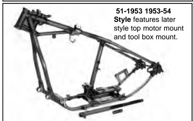
**51-1953 1953-54 Style** features later style top motor mount and tool box mount.
