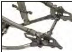
**Seat Area** utilizes cast yoke to accept stock seat post bushing which is included. Rear down tube has cast front oil tank mount and coil mount blocks installed. Lower tube bushing is welded to secure lower seat post lock nut.
