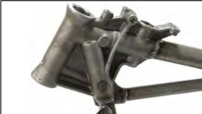
**Rear Section** demonstrated forged rear axle plates and replica tool box mount for authentic look.
