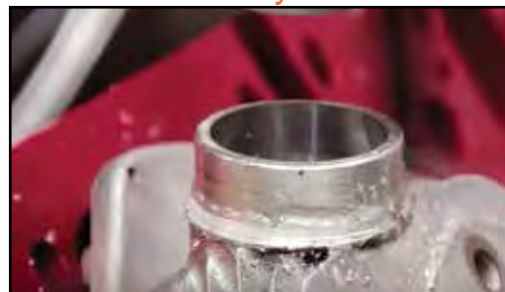
Motor Shop Exhaust Port Replacement
