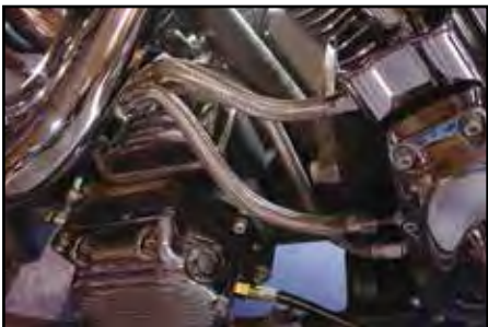
Custom Stainless Steel Oil Line Kit fits TC-88 for custom applications. Includes three compression fittings and three seal ends. Hose must be cut for installation. VT No. 40-0467
