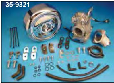
**Mikuni HSR42/45 Total Kit** for Big Twins. These kits are complete with all required parts for installation. Kits include HSR 42mm or 45 mm carburetor, intake manifold, rubber flange, K&N filter, chrome cover, breather kit and mounting hardware. Models from 1990-up use stock throttle/idle cables and 1984-89 models require 1990-up cables.
