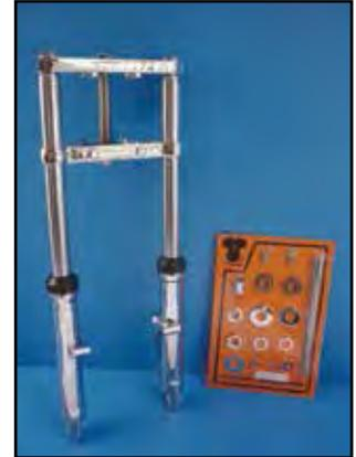
**FXST Style Single Disc Fork Assembly** features chrome trees with 1" stem, polished or chromed lower slider legs, to accept 11.5" caliper and brake disc, hard chrome fork tubes, axle, neck bearings, top cone and stem nut, pinch bolts and bearing dust covers. Fork is 31" overall length (L) and legs are assembled. Single disc unit accepts 11.5" brake disc and left side caliper.
