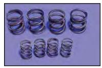
Valve Springs include inner and outer as required. Fits 1984-04 Big Twin Evolution/TC-88. Replaces OEM 18201-83.
