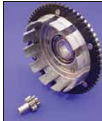
Easy Starter Kits for Big Twin Models. Improves starting on high compression big inch engines through an improved starter-to-clutch basket gear ratio. Complete kits include a clutch basket with bearing for Big Twin models with 66-tooth starter ring and a 9-tooth starter pinion gear.
