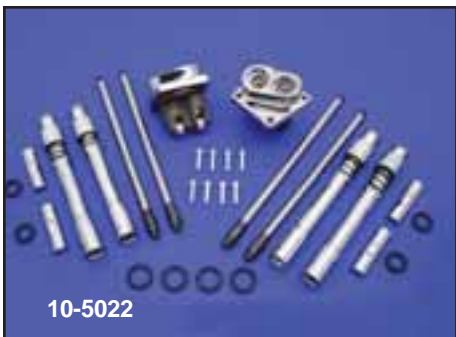
Velva Touch Hydraulic Lifter Kits for Evo feature solid tappet performance with hydraulic tappet convenience. The patented design replaces aluminum tappet blocks with a cast iron alloy, and with tappets that each have their own independent oil supply for improved lubrication and enhanced tappet operation. Kits include tappets, chrome tappet blocks, pushrods, pushrod covers, bolts and seals. Stroker pushrods are .250" longer than standard. For use with cams up to .640 lift.
