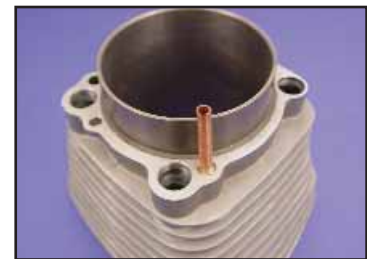
VT No.16-0911 Tube Installed
