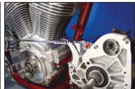
Billet Shift Arm fits 5 & 6 Speed Big Twin transmissions. VT No. 17-0666
